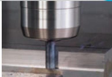
GS MILL高硬圆角型的SKD61(53HRC)侧面加工
