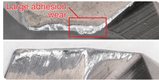
After drilling 900 holes
