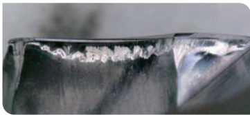
After drilling 46m
