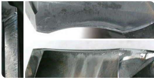
After drilling 2,500 workpieces (5 holes per workpiece)
