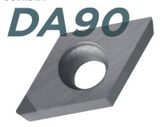
A polycrystalline diamond grade in which coarse diamond particles have been sintered to form a dense structure. The high diamond content, with high wear resistance, makes it ideal for roughing of cemented carbide and hard brittle materials.
