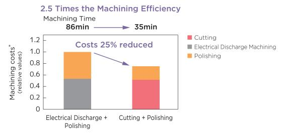
\*Assuming  $\emptyset 4.0 \rightarrow \emptyset 4.5 \times L20$  turning with machining costs at 3,500 JPY/h, calculating tool life at 30 units/pc
