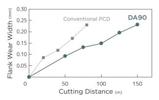
Work Material: Cemented Carbide VC50 (87HRA) Tool: NF-DCMW070204 Cutting Conditions: vc = 20m/min f = 0.1mm/rev ap = 0.2mm Wet
