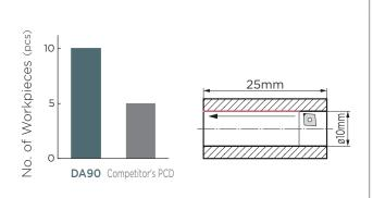
Tool: NF-CCMW04X102 (DA90) Internal Boring Cutting Conditions: vc = 20m/min f = 0.075mm/rev ap = 0.1mm Wet
