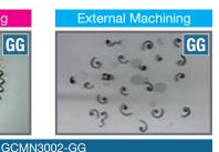
Chip shapes differ between internal machining and external machining even under the same cutting conditions.
