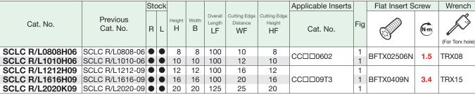
When using handed breaker inserts for facing, the holder and insert are opposite handed.
