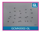
Work Material: SCM415 Prepared Hole Diameter:  $\emptyset$ 25mm Holder: GNDI R2532-T306 Insert: GCM N300 $\bigcirc$ - $\bigcirc$  Cutting Conditions:  $\forall c = 100 \text{m/min}$ , f = 0.1 mm/rev, ap = 3.0 mm Wet
