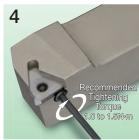
Tighten the shim set screw. (Recommended Tightening Torque 1.0 to 1.5N·m)
