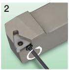
Loosen the shim set screw by one to two turns.
