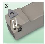
Remove the shim and attach a different shim that matches the lead.
