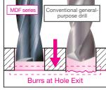
Work Material: SCM415 Machine: BT40 Vertical Machining Centre Tool: MDF 0500S2D (ø5.0mm x 2D) Cutting Conditions: VC = 65m/min, f = 0.12mm/rev, H = 10mm. 150 holes, Wet
