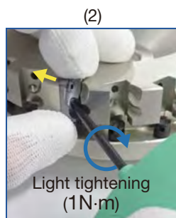
(2) Lightly tighten the cap screw while pressing the blade against the restraining face. (1N·m)
