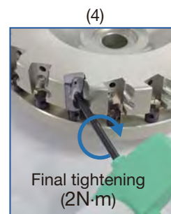
(4) Perform final tightening of the cap screw. (2N·m)
