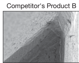
Chipping in edge coating
