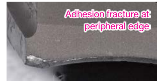
Competitor's Product C after 40m of drilling
