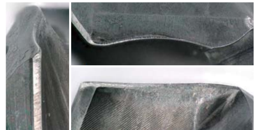
MDM series after 200m of drilling
