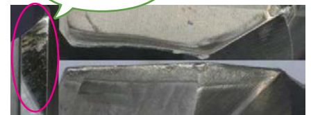
Cutting Conditions: f = 0.60mm/rev Cutting Length: 60m (drilling time 39 minutes)
