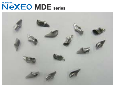
Chips are broken into small pieces
