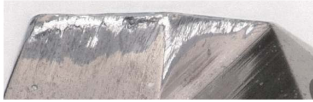
After drilling 900 holes
