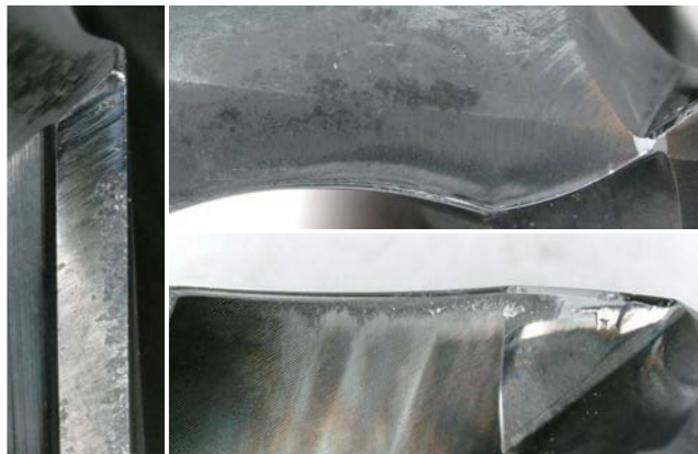
After drilling 2,500 workpieces (5 holes per workpiece)
