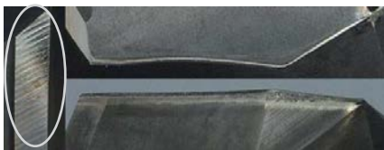
Cutting Conditions: f = 0.30mm/rev Cutting Length: 30m (drilling time 39 minutes)
