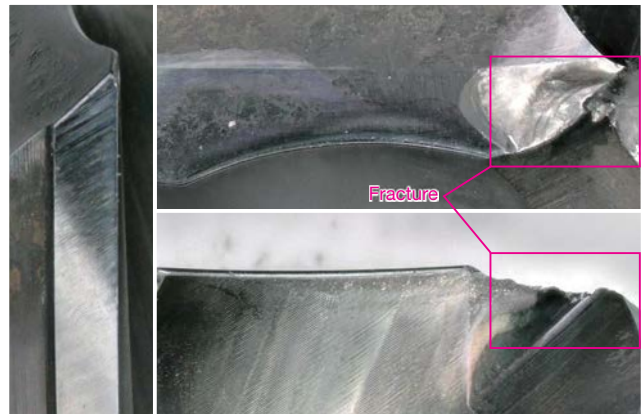
After drilling 1,000 workpieces (5 holes per workpiece)
