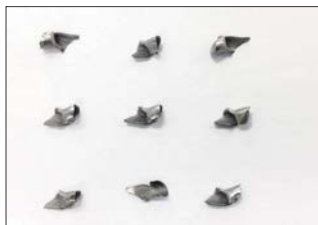
Chips are broken into small pieces
