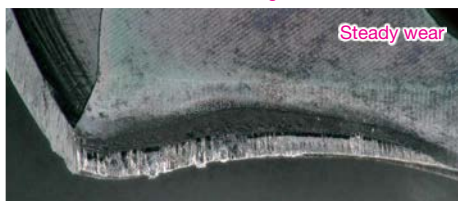
MDM series after 80m of drilling
