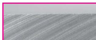
SUMICRYSTAL (Single-crystal Diamond) SC10 Wiper Blade Machined Surface
