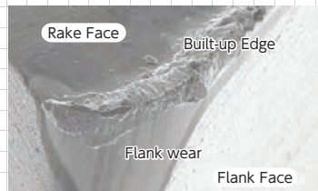
工具の摩耗と構成刃先 Flank wear and built-up edge
