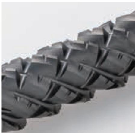
Variably sized nicked cutting edge shape realises stable machining with low resistance
