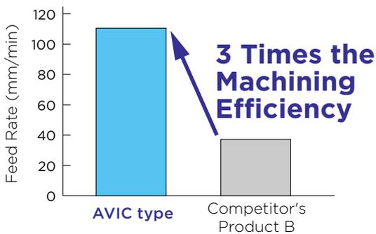
AVIC type has 3 flutes for higher-efficiency machining
