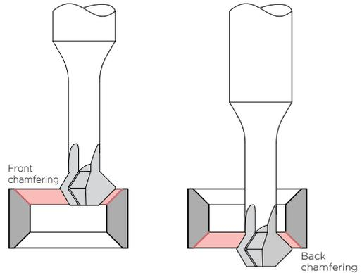
Front and back chamfering is possible with a single tool
