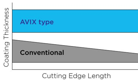
Uniform coating thickness realises stable tool life
