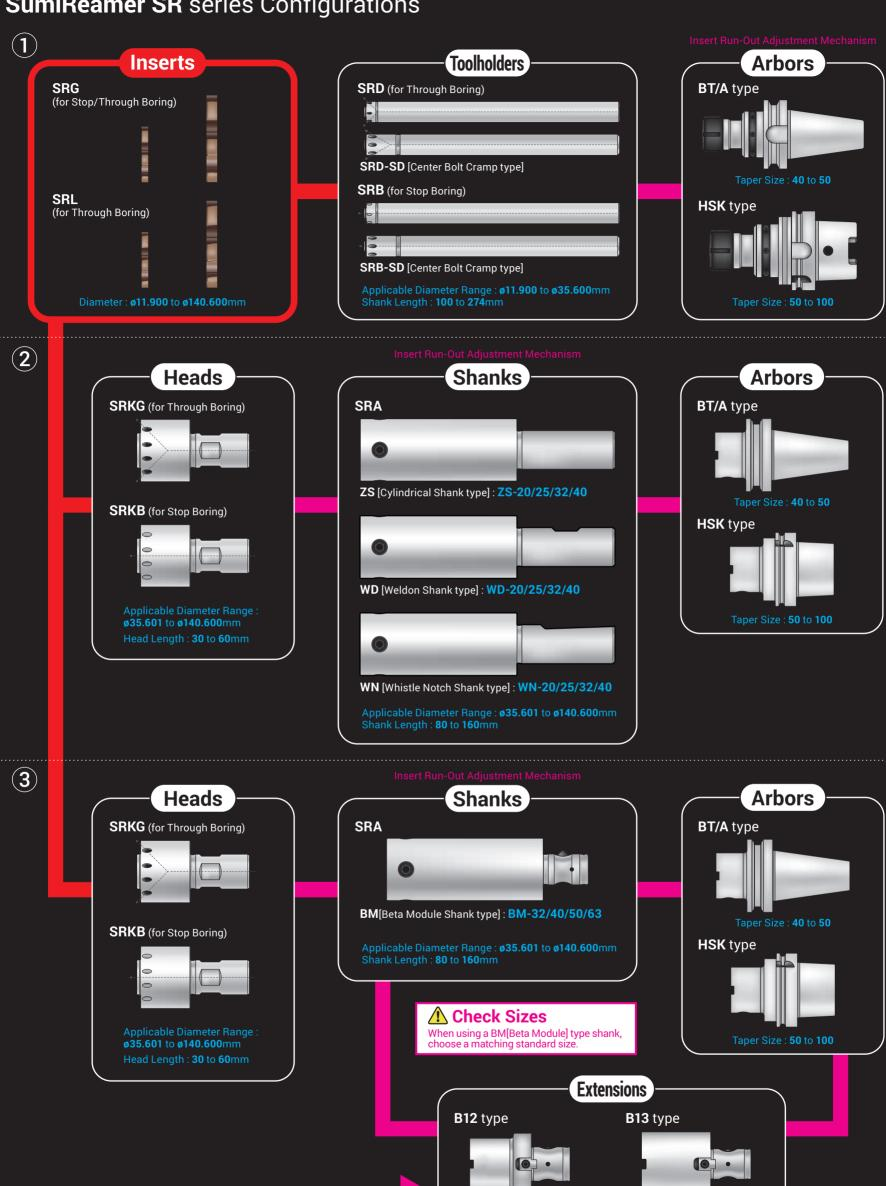
Multiple extensions can be connected together When connecting multiple extensions, it is recommended to consider rigidity and use longer shank sizes so that the total number of extensions is as low as possible.
