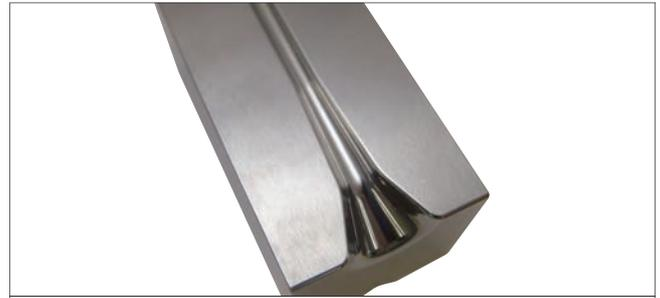
Work Material : Cemented Carbide VF20 (Ultra-fine Grain AF1, 92.5HRA)
