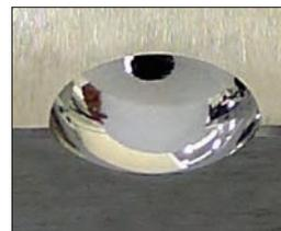
Mirror finishing of Cemented Carbide
