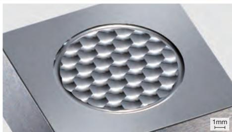
Work Material : Cemented Carbide VF20 (Ultra-fine Grain AF1, 92.5HRA)
