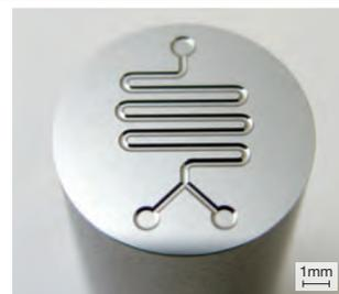
Work Material : Cemented Carbide VF20 (Ultra-fine Grain AF1, 92.5HRA)
