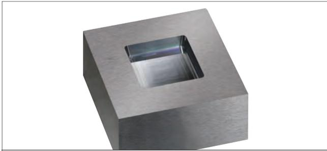
Work Material : Cemented Carbide VF20 (Ultra-fine Grain AF1, 92.5HRA)
