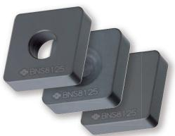
Optimising the particle size distribution of the CBN particles has resulted in improved chipping resistance and longer life while maintaining wear resistance during grey cast iron machining
