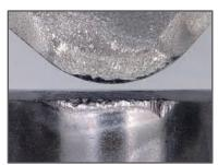
Conventional Tool (Uncoated) (After Cutting 9.0km)
