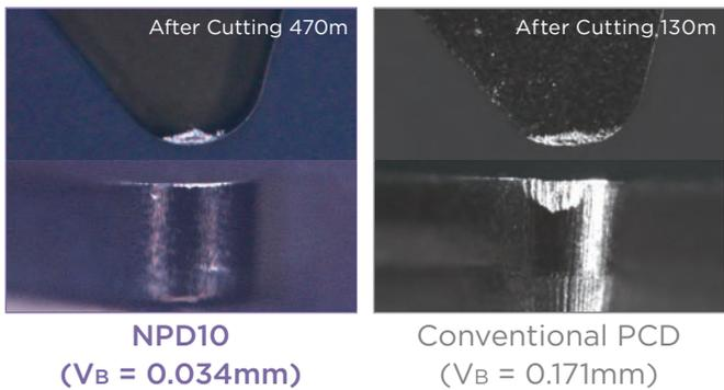
Work Material: Cemented Carbide (87HRA) Tool: DCMW11T304RH
