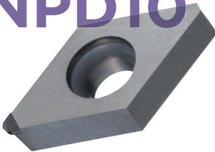
Cutting edge is 100% diamond material made from high-hardness nano-crystalline diamond which, unlike single-crystal diamonds, has no anisotropy. Achieves longer tool life and higher machining accuracy than conventional diamonds in the machining of cemented carbide and other hard brittle materials.
