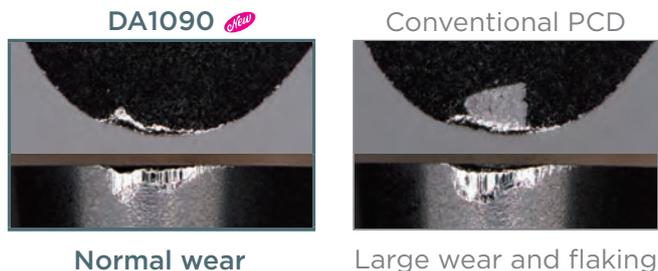
Work Material: Cemented Carbide VM30 Equivalent (91HRA)
