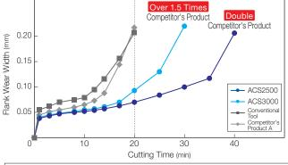
$\label{eq:machine} \begin{tabular}{lll} Machine & : Vertical Machining Centre BT40, Work Material: Ti-6Al-4V \\ Tool & : RSE 12050RS05, Insert: RPHT1204M0EN-G \\ Cutting conditions : $v_c = 70 m/min f_z = 0.25 mm/t $a_p = 2 mm $a_e = 30 mm$ Wet \\ \end{tabular}$
