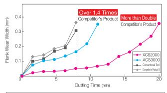
$\label{eq:machine} \begin{tabular}{ll} Machine &: Vertical Machining Centre BT40, Work Material: Inconel 718 (44HRC) \\ Tool &: RSE 12050RS05, Insert: RPHT1204M0EN-G \\ Cutting conditions &: $v_c = 40 m/min f_z = 0.3 mm/t a_p = 2 mm a_g = 30 mm \end{tabular}$
