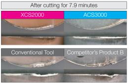
Superb fracture resistance for a tool life 1.4 times greater than that of conventional tools and competitor's products
