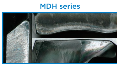
After Drilling 1,500 pcs
