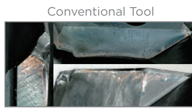
After Drilling 500 pcs
