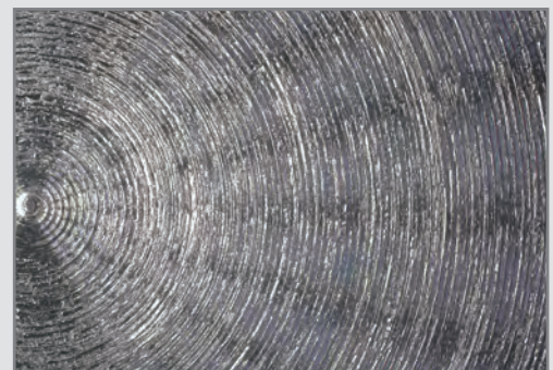
Machined surface ( v_c = 100\text{m/min} or below)
