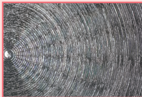
Machined surface ( v_c = 100\text{m/min} or below)
