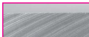
SUMICRYSTAL (Single crystal diamond) SC10 wiper insert machined surface
