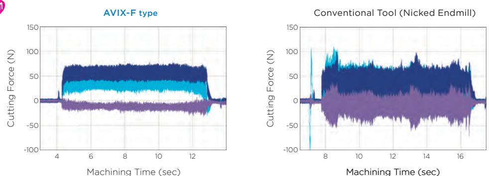
Work Material: CFRP (Thickness 2mm)
