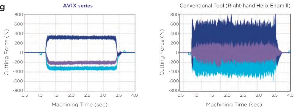
Work Material: CFRP (Thickness 9.5mm)
