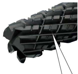
Main cutting edge (upward force) and sub-cutting edge (downward force) form a complex cutting edge shape which suppresses work material vibration
