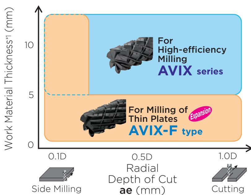
\*1: Recommended work material thickness at cutting is 1.0D or below for AVIX series and 0.5D or below for AVIX-F type
