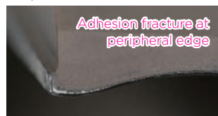
Competitor's Product A after 80m of drilling
