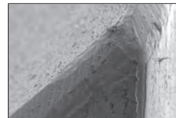
Chipping in edge coating
