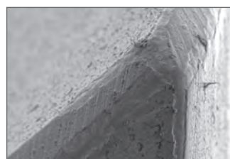
Chipping in edge coating
