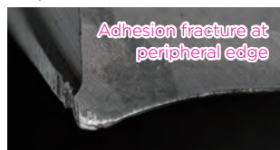
Competitor's Product B after 80m of drilling
