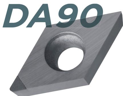
A polycrystalline diamond grade in which coarse diamond particles have been sintered to form a dense structure. The high diamond content, with high wear resistance, makes it ideal for roughing of cemented carbide and hard brittle materials. Optimised design and mass production technology have been developed, achieving the same performance as conventional tools with higher cost-performance.
