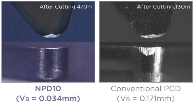
Work Material: Cemented Carbide (87HRA) Tool: DCMW11T304RH
